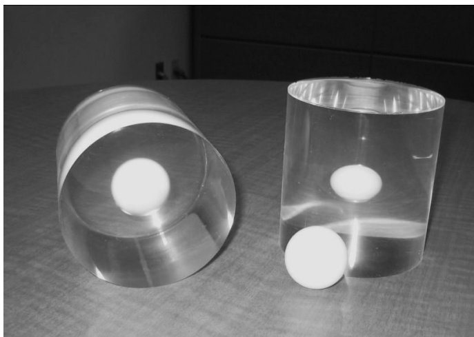
Fig. 1: C-1025 Volumetric CT Resolution Phantom
